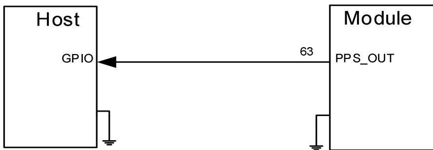
Figure 4.15 1PPS Output Interface Reference Circuit
