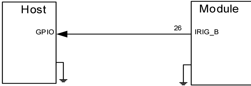
Figure 4.14 B-code output interface reference circuit
