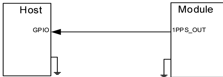
Figure 4.16 1PPS Output Interface Reference Circuit
