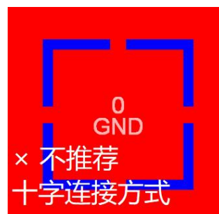
Figure 5.4 Non-recommended copper laying method
